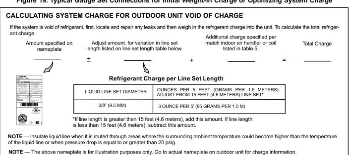
Figure 20. Using HFC-410A Weigh In Method
